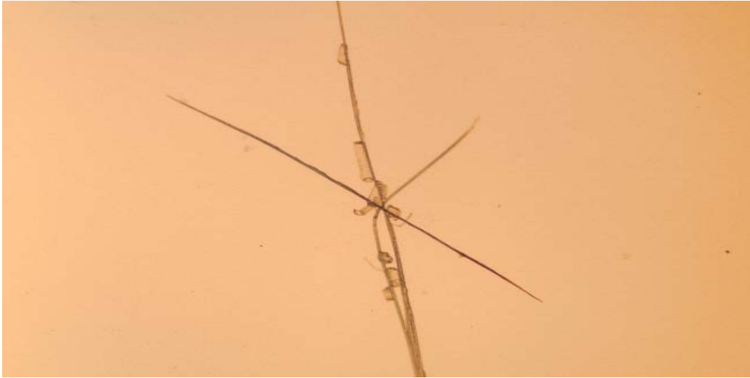
Figure 3-4. A view of the macerated bamboo fibers under microscope (20 × magnified).
