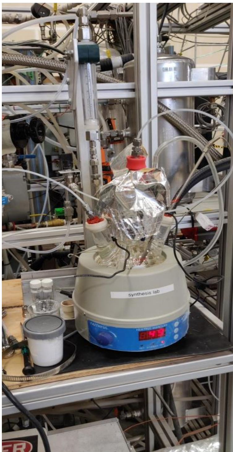
Fig. S3 Test rig for flue gas exposure of CALF20 from a natural gas burner.
