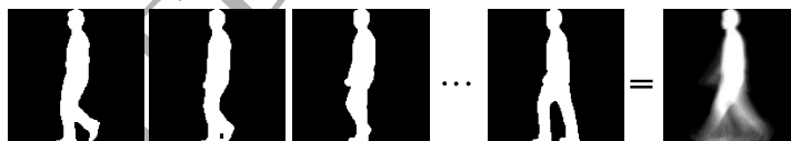
Figure 2: Gait energy image (the right one) is produced by averaging the silhouette in one gait cycle.
