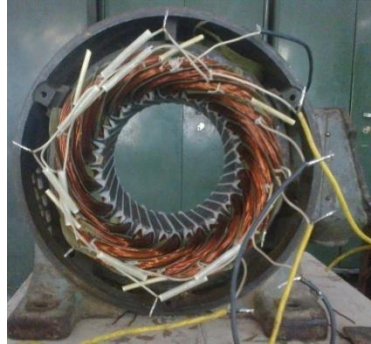
Fig. 2 Stator of Induction Motor
