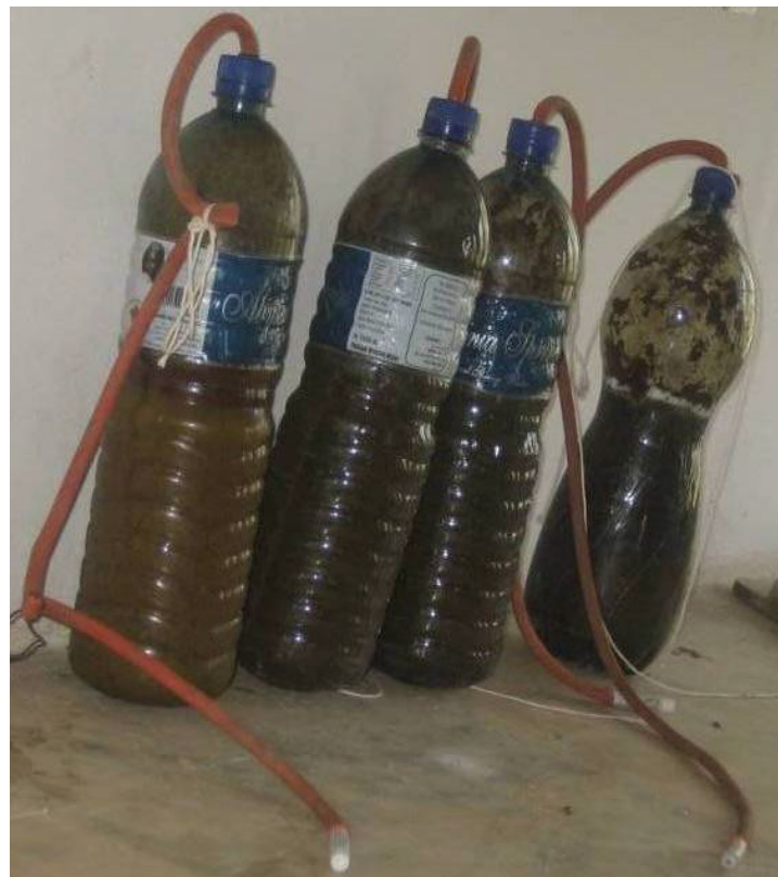
Figure 3. Pilot scale anaerobic digesters of 1.8 L volume
