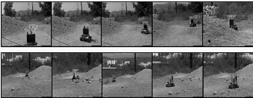
Figure 11.17: Navigation Path using Strategic Navigation Behaviors. Top-left Image Shows the Initial Position; Bottom-right Image Indicates Goal Achievement.
