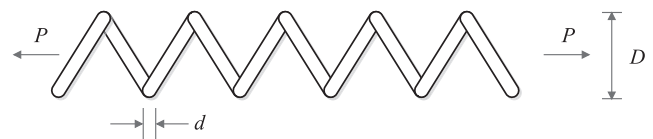
Fig. 20. Schematic view of tension/compression spring problem.
