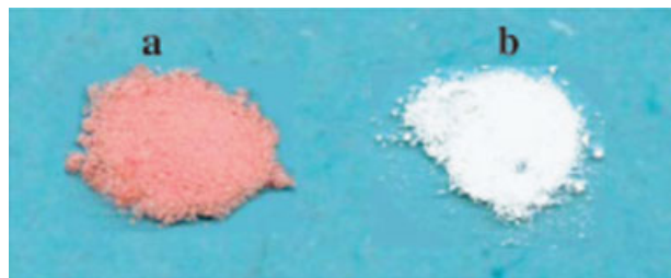
Figure 5. Picture of PMMA synthesized by the RAFT process (a) before and (b) after the reaction with AIBN at 80 °C for 2.5 h.
