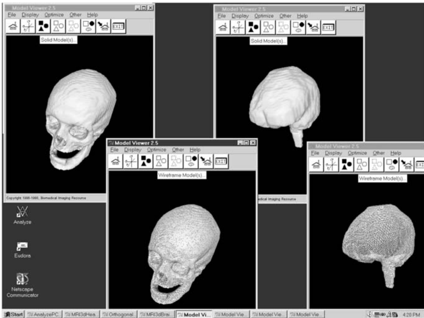
FIGURE 5 Shaded surface displays of segmented skull and brain (top left and right, respectively) with underlying polygonal representations (bottom).
