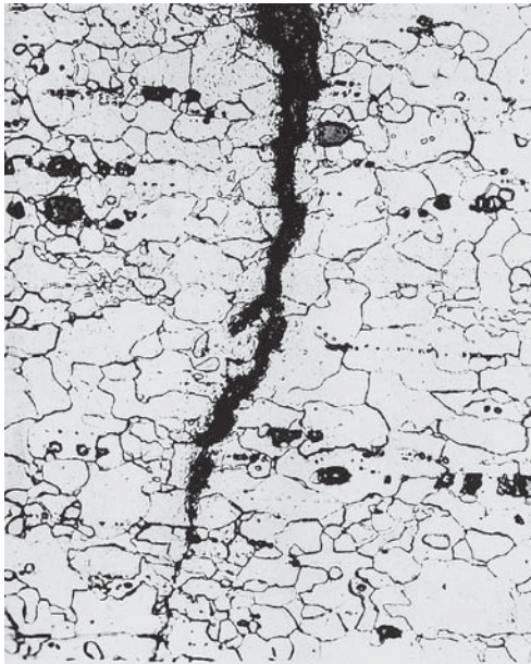
Figure 8.16. Corrosion-fatigue crack through mild steel sheet, resulting from fluttering of the sheet in a flue gas condensate (250 \times ).
