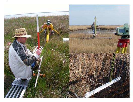
**Figure 6.23.** Examples of techniques for leveling to the top of deployed SET instruments. Left panel: digital barcode leveling. Note rod level against invar strip (rod) to keep rod plumbed. Top right: Two meter level rod placed on top of a first generation SET. Note that rod is placed near the base; additional measurements are needed to transfer elevation differences to the SET plate. Bottom right: digital barcode invar strip on RSET arm.
