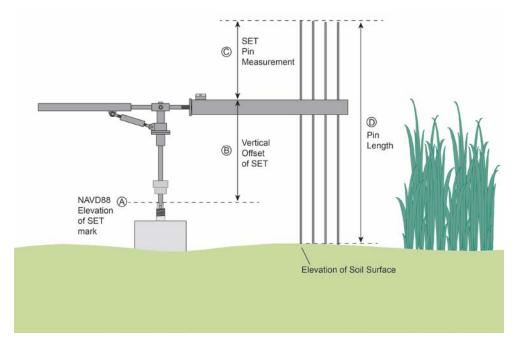
**Figure 6.22.** Diagram displaying steps involved in transferring elevation of an SET mark to individual SET pin observations (not all pins shown).
