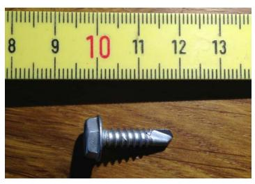
Figure 3.30. Self-tapping screw (metric ruler above).
