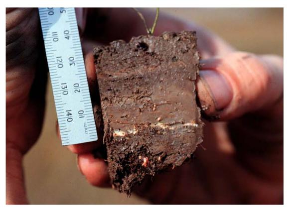
Figure 5.38. Measuring a cut plug core. Note the thin feldspar marker horizon.
