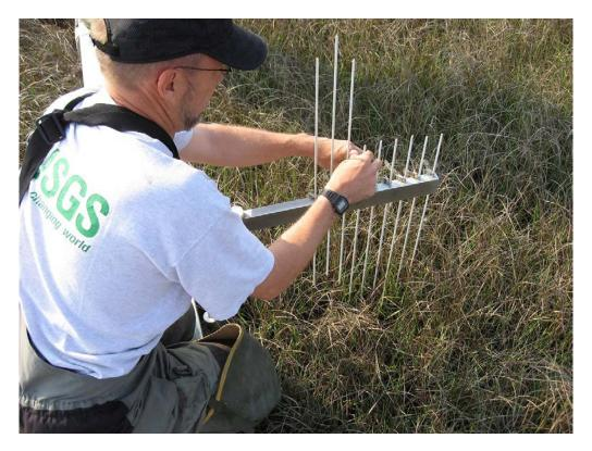
Figure 4.17. Lowering pins to the surface (Blackwater NWR, MD USA).
