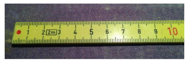
Figure 5.17. Metric ruler (note that it starts at zero).
