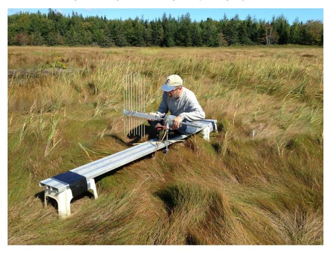
**Figure 2.20.** Temporary platform (Acadia National Park, ME, USA). Note the step stools are attached to the plank with duct tape.
