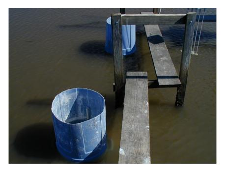
**Figure 5.6.** Feldspar marker horizon plots established using trash cans in a shallow pond with about 8" (20 cm) of water (Delta NWR, Venice, LA USA).
