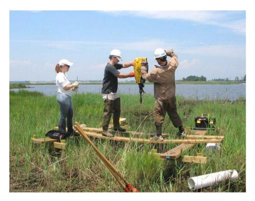
Figure 3.5. Gasoline powered hammer drill (Chesapeake Bay Environmental Center, MD, USA).
