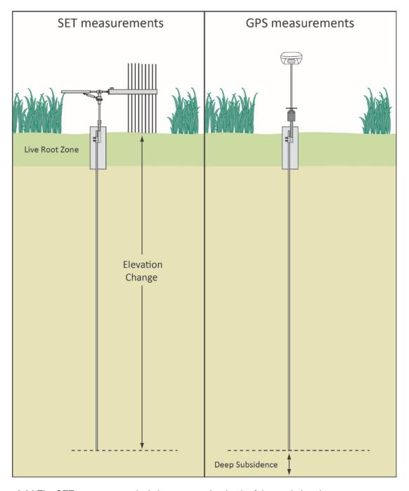
**Figure 6.24.**The SET measures vertical change over the depth of the mark, but does not measure processes occurring below the mark, such as uplift or subsidence (left panel). Repeated GPS measurements on top of the SET mark can be used to monitor processes occurring below the mark (right panel).
