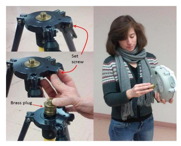
**Table 6.7.** Removing the threaded brass plug at the top of a Fixed Height GPS tripod and threading into the base of a GPS antenna.
