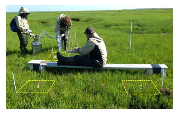
**Figure 5.32.** Sample station showing the three feldspar plots (dashed yellow lines). Note the corners of the sample station are marked with taller fiberglass stakes. Not all stakes are visible (Assateague Island NS, MD, USA).
