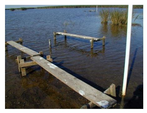
**Figure 2.5.** A permanent platform in a shallow pond (Delta NWR, Venice, LA, USA) with an original pipe SET mark. Note the mark is raised above the water to accommodate the SET, which requires longer SET pins to reach the water bottom.
