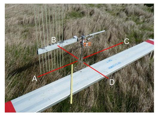
**Figure 4.10.** Rod SET on a deep rod mark showing the 4 directions measured (note: the Direction A stake is hidden by the vegetation an plank and is not visible in the photograph).
