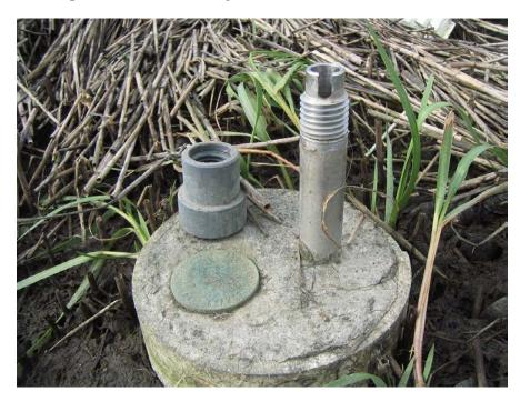
**Figure 4.13.** A receiver with cap removed showing the notch in the receiver; and the brass marker used to ID the SET mark
