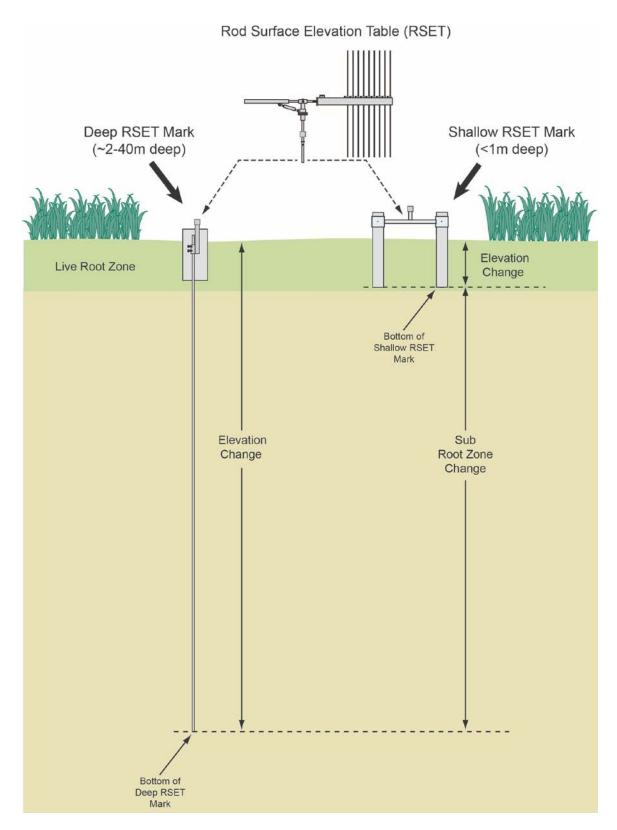
**Figure 3.1.** Cross section of a wetland showing the deep and shallow RSET marks commonly used for monitoring elevation change. The deep mark consists of 4 foot (1.2 m) sections of stainless steel rod threaded together.
