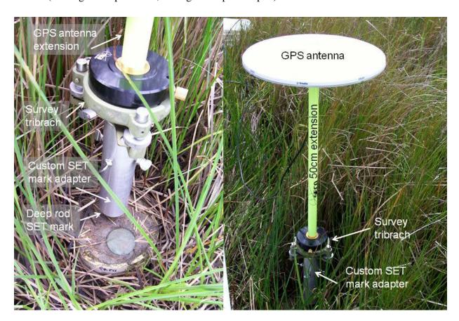
**Figure 6.11.** Custom adapter used to place a GPS antenna on a deep rod SET mark for a static GPS occupation.
