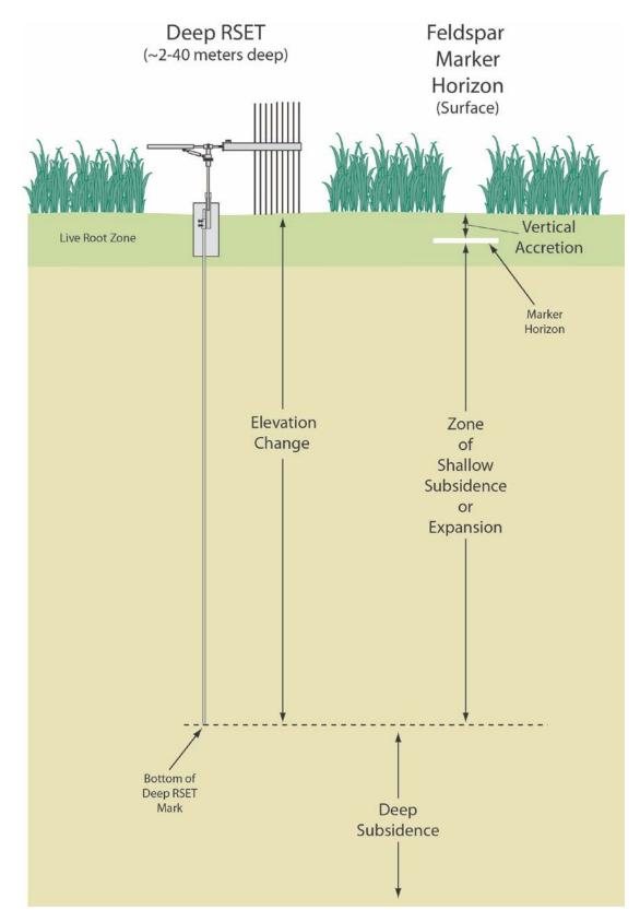
**Figure 9.** The combined Surface Elevation Table – Marker Horizon technique enables estimates of both above and below-ground process contributions leading to wetland elevation change.
