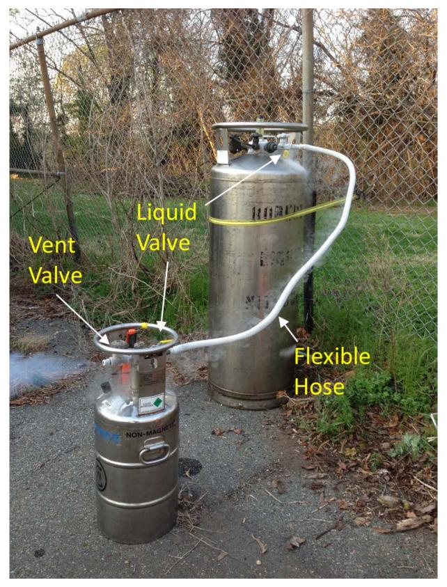
**Figure 5.30.** Filling a 15 L dewar from a larger tank. Note the white exhaust coming from the vent, which is normal.
