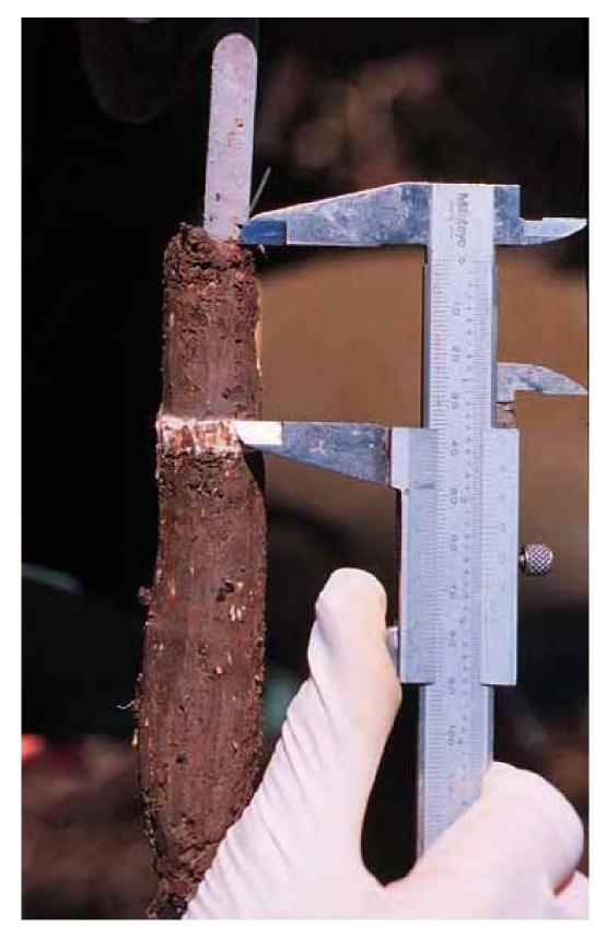
Figure 5.37. Measuring a frozen sediment core (cryo-core) showing the feldspar marker horizon.
