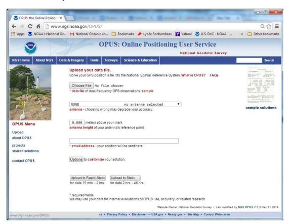
Figure 6.15. Sample OPUS GPS processing upload page, showing required input fields.
