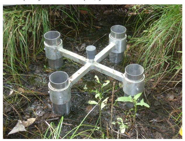
**Figure 3.35.** Completed installation of a shallow SET platform. Note that the legs are now attached to the framework with screws.
