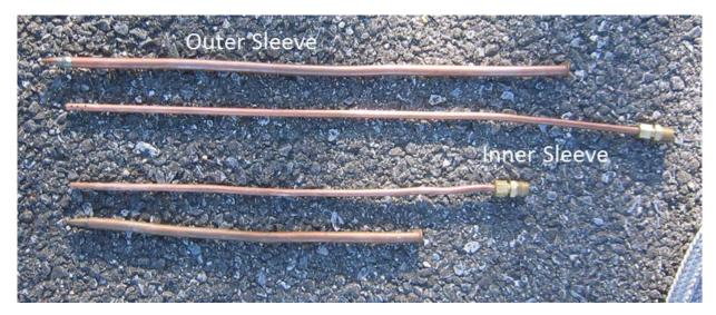
Figure 5.18. The "Bullet": The inner sleeve and the outer sleeve.
