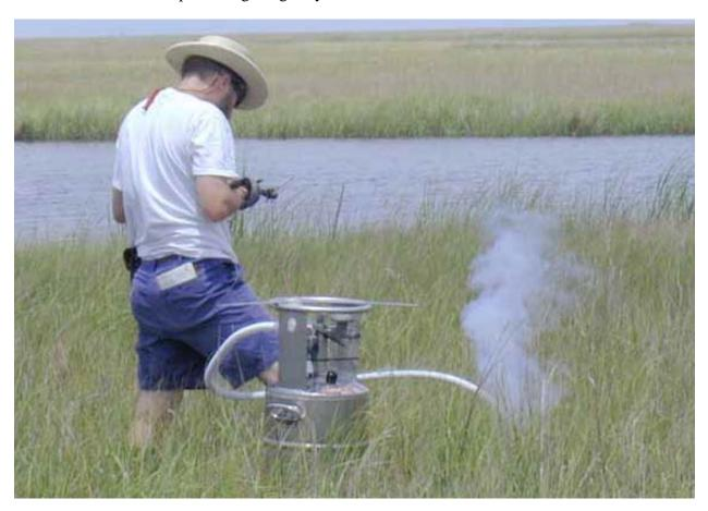
**Figure 5.34.** Taking a cryo-core. Note white cloud from the LN<sub>2</sub> escaping the bullet (Fire Island NS, New York, NY USA).
