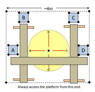
**Figure 2.7.** Schematic showing the sample station layout when using a permanent platform with teeth. Note that the two parallel planks are typically permanent and the middle plank is only deployed during measurements.
