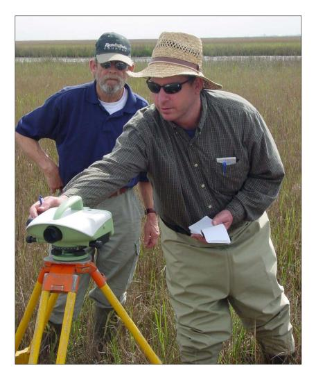
Figure 6.19. Leveling in the wetland: Operator(s) standing away from tripod, while activating electronic measurement.
