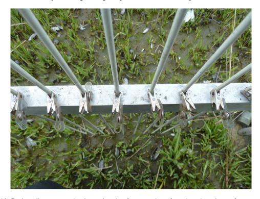
Figure 4.16. Badge clips are used to keep the pins from moving after placed on the surface.
