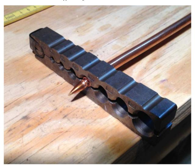
Figure 5.26. Compress the copper tube and bullet.
