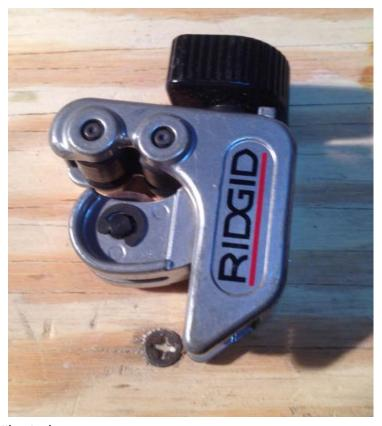
Figure 5.21. Pipe cutting tool.
