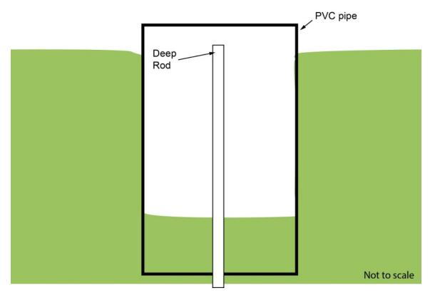
Figure 3.18. PVC collar in the ground.
