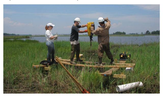
**Figure 23.** Installing a deep RSET mark in a Chesapeake Bay brackish marsh. In this example, a portable gasoline powered jackhammer is being used to drive rods. Note the permanent sampling platform installed to minimize human disturbance of the marsh surface where the readings will be taken. A removable, portable platform could also be used (Chesapeake Bay Environmental Center, MD, USA).
