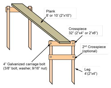
**Figure 2.8.** Detail of one side of an SET platform, showing approximate dimensions of the component parts.
