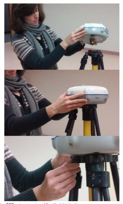
Figure 6.8. Placing GPS antenna on top of fixed height tripod.
