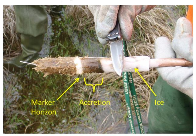
**Figure 5.35.** Scraping a frozen core. Marsh was covered in water which froze during coring (Gateway NRA, New York, NY USA).
