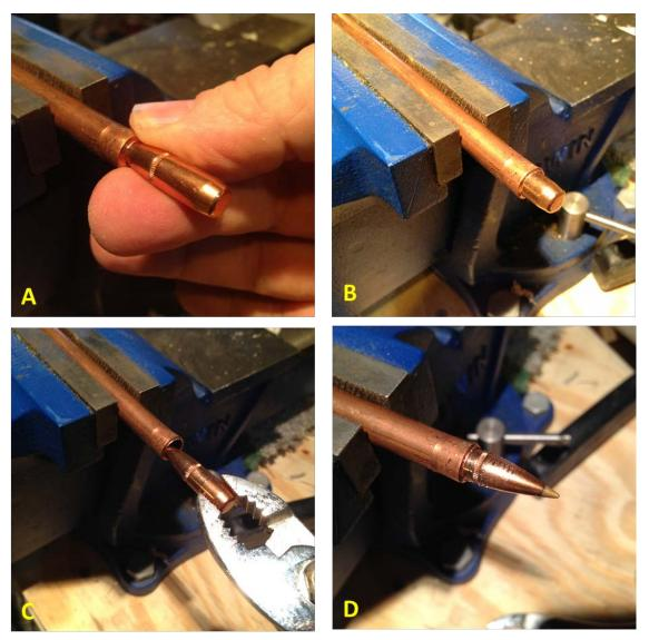
**Figure 5.25.** How to open up the end of the outer sleeve to insert the bullet. A) Place bullet "tip first" into the copper tube (use a vice to hold the sleeve), B) Tap the bullet into the copper tubing with a hammer, C) Remove the bullet with pliers, D) turn bullet around and place into the copper tubing. The bullet is now ready for soldering.
