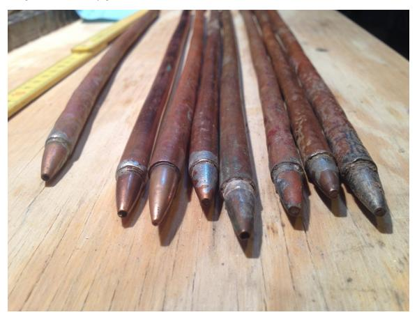
Figure 5.16. Copper bullet probes (outer sleeves).
