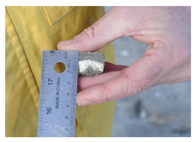
Figure 5.40. Cut plug core at a marsh restoration site.
