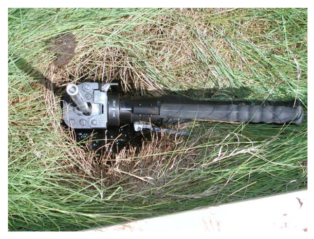
Figure 3.17. Hydraulic bolt cutter attached to the deep rod.
