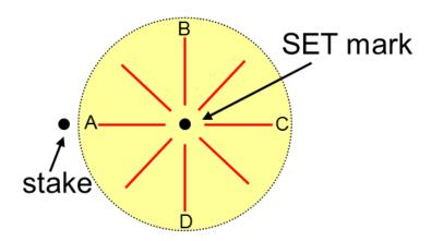
**Figure 4.9.** A method for identifying the orientation of SET measuring directions using a single stake to indicate direction A. Only the ABCD directions are measured in this example, which is typical for most sample stations.
