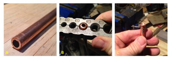
Figure 5.24. Flaring the outer sleeve of the bullet.
