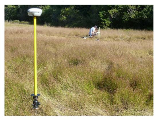
**Figure 25.** GPS receiver deployed on an SET mark for a static occupation (Acadia National Park, ME, USA).
