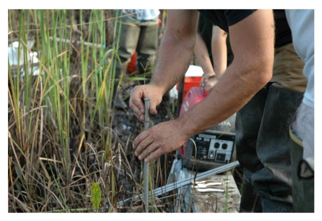
Figure 3.10. Attaching the driving head (Waccamaw River, South Carolina, USA).
