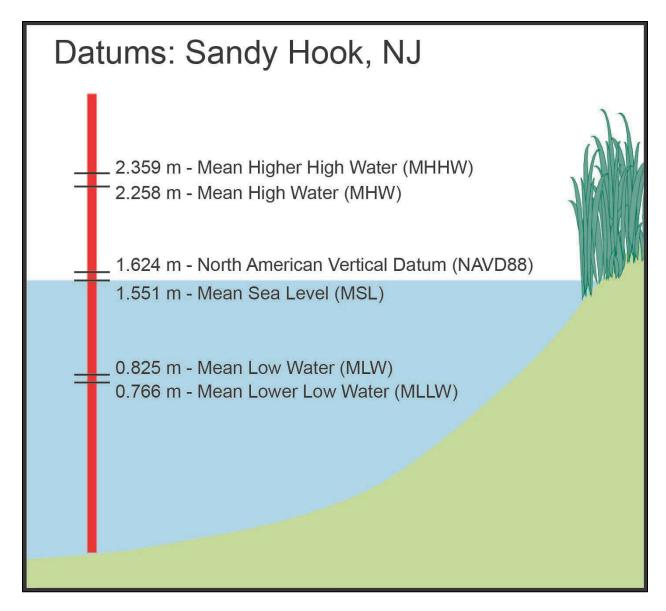
**Figure 10.** Schematic showing the vertical relationships among tidal datums at a tide station. All values are given with respect to the (arbitrary) local station datum. Note the reference to the orthometric datum, NAVD 88 is also given (source: NOAA Center for Operational Oceanographic Products and Services).
