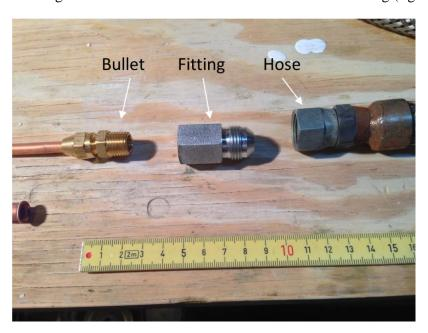
Figure 5.15. Fittings for bullet probe and hose.
