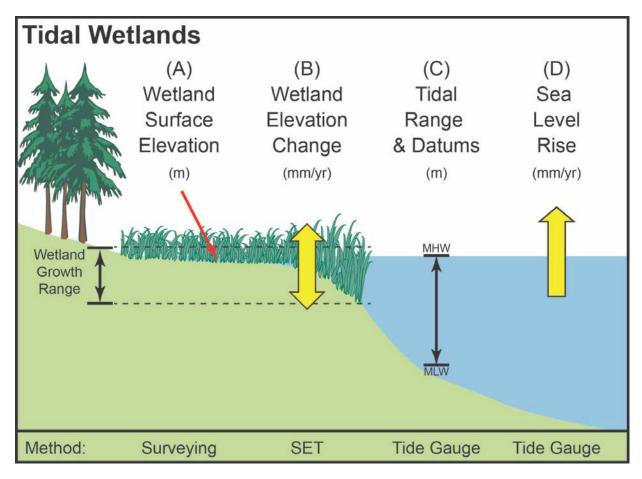
**Figure 2.** Conceptual diagram showing the relationship among wetland surface elevation (A), tidal datums (C), and their respective rates of change (B and D). Understanding these relationships is important for evaluating the sustainability of a wetland community to sea-level rise.
