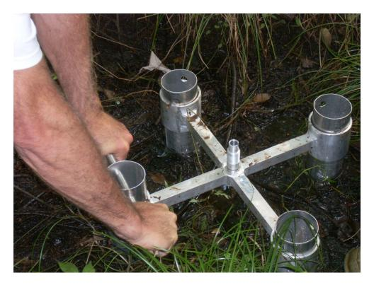
Figure 3.33. Twisting the last leg of the platform into the soil.
