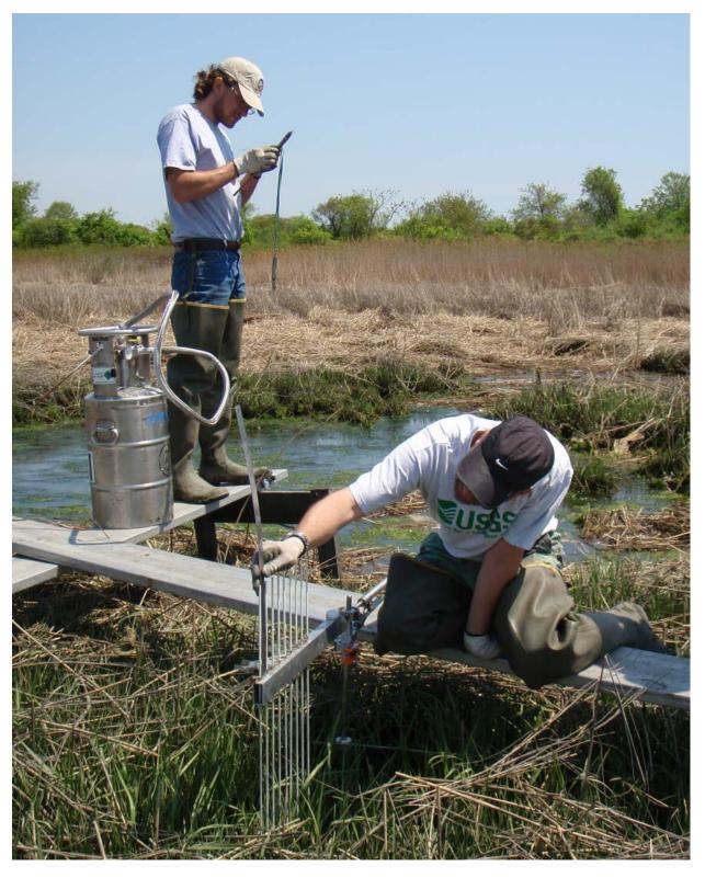
**Figure 5.36.** SET measurements and cryogenic coring on a permanent platform (Gateway NRA, New York, NY USA).
