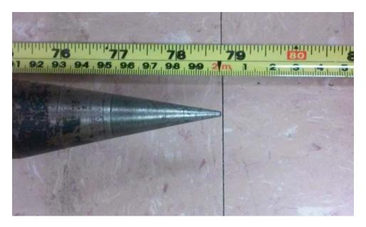
Figure 6.6. Verifying the length of the central leg of a fixed height GPS tripod.
