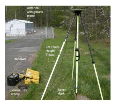
**Figure 6.13.** GPS antenna with ground plane atop a two meter fixed-height tripod. Note that in this case the GPS receiver is a separate unit, connected to the antenna via a coaxial cable. Also note external power source (12 volt automobile battery) to ensure uninterrupted power during long observations (in this case, up to 12 hours).
