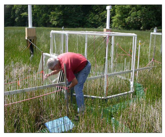
**Figure 15.** The Smithsonian Institution's "Monster SET" in operation. The RSET instrument, with a 4 meter long arm incorporating 100 pins, is able to cross both treatment (CO<sub>2</sub> enclosure = PVC structure) and control areas outside the treatment enclosure (Smithsonian Environmental Research Center, MD, USA).
