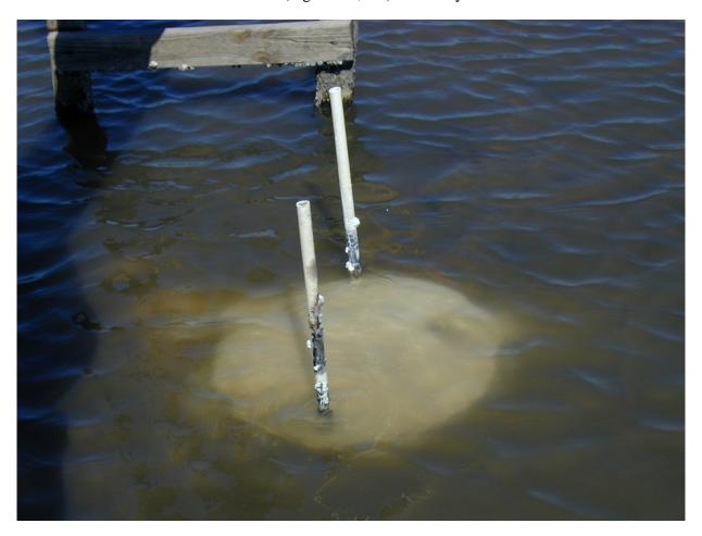
Figure 5.7. Feldspar marker horizon after removing the trash can (Delta NWR, Venice, LA USA).
