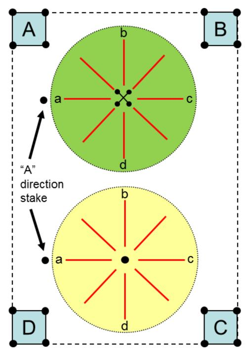
**Figure 2.3.** Sample station layout with a shallow and deep mark and marker horizons. Yellow circle = Deep RSET mark measuring area, Green circle = Shallow RSET Mark measuring area, Blue boxes = Marker horizons, Black circle = stakes.
