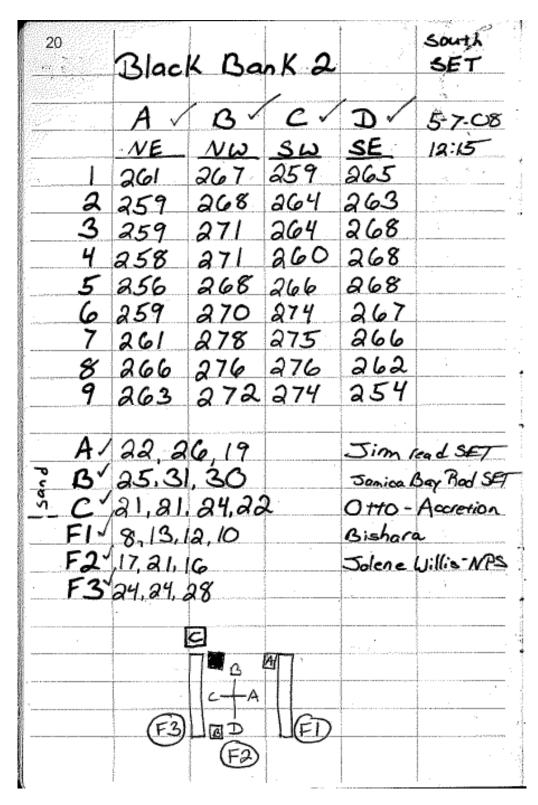
**Figure 29.** Typical SET-MH data book entries as recorded in the field. Note date, sample site and station ID, SET positions, pin numbers, pin heights and sample station sketch.
