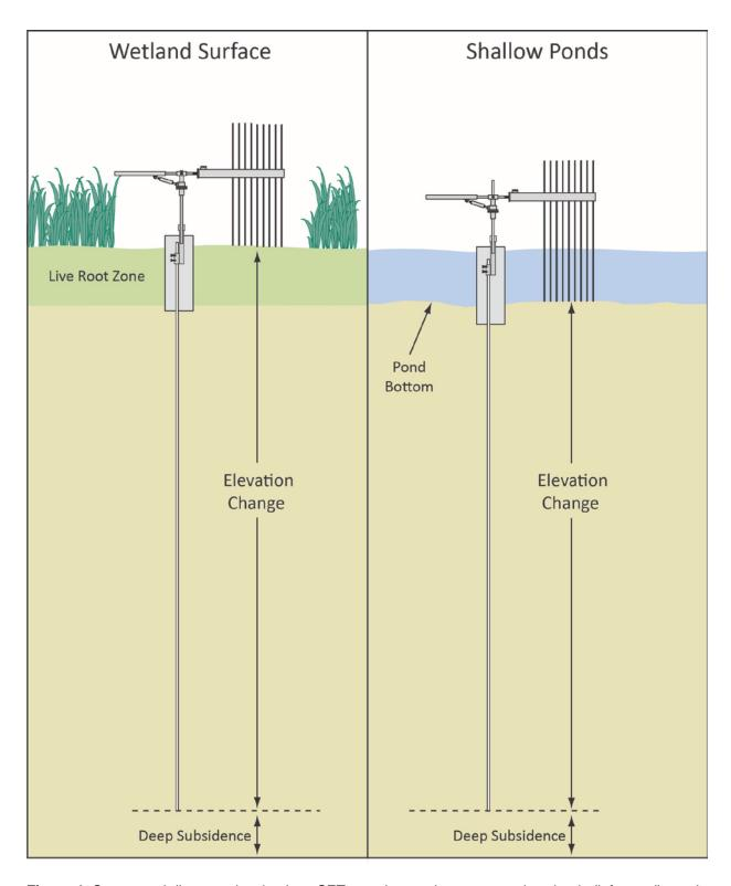
**Figure 4.** Conceptual diagram showing how SETs can be used on vegetated wetlands (left panel), mud flats and shallow ponds (right panel). In both cases, a deep RSET mark is established in the soil and the pins are placed on the sediment surface. The SET measures relative elevation change occurring from the base of the SET mark to the sediment surface. Relative elevation is measured as the height of the pins above the horizontal arm of the SET.
