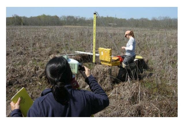
**Figure 26.** Digital barcode leveling is used to transfer elevations from a SET mark to other vertical infrastructure (Jug Bay, MD USA).
