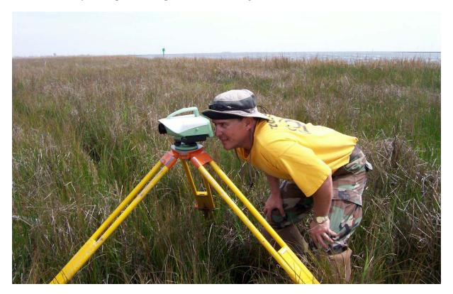
Figure 6.18. Leveling in the wetland: note splayed legs of tripod to enhance stability.
