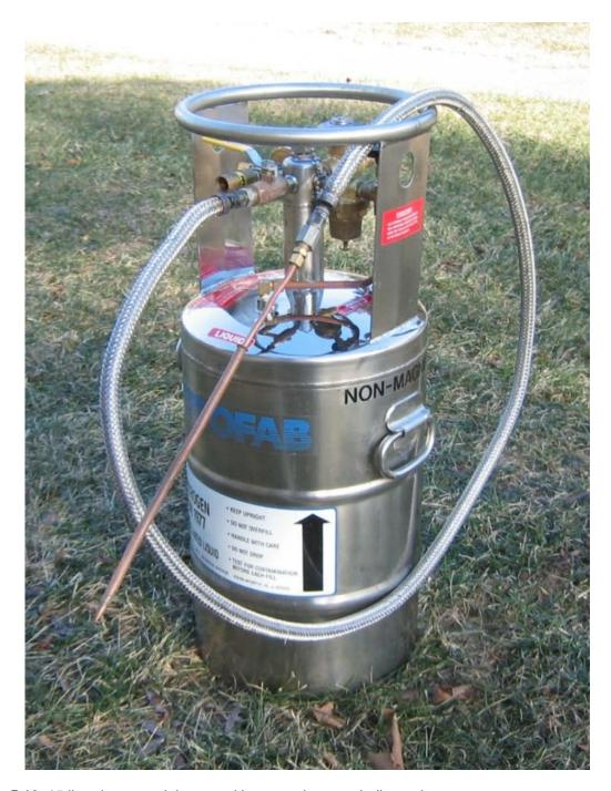
Figure 5.10. 15 liter dewar, stainless steel hose, and copper bullet probe.
