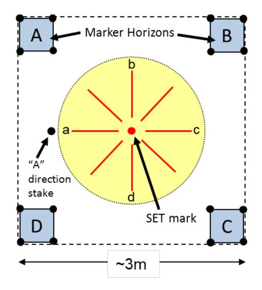
**Figure 2.2.** Sample station layout showing a single deep RSET mark and four marker horizons and the 8 potential directions for measurements. Yellow circle = SET measurement area, Blue boxes = marker horizons, Black circle = stakes (not to scale), Red line = Potential direction for measurement.
