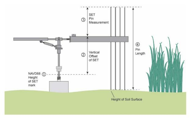
**Figure 27.** Diagram displaying data involved in transferring elevation of an SET mark to individual SET pin measurements (not all pins shown).
