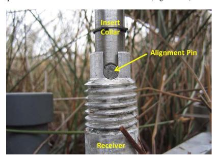
Figure 4.14. The base of the RSET instrument connects with the receiver using an alignment pin.
