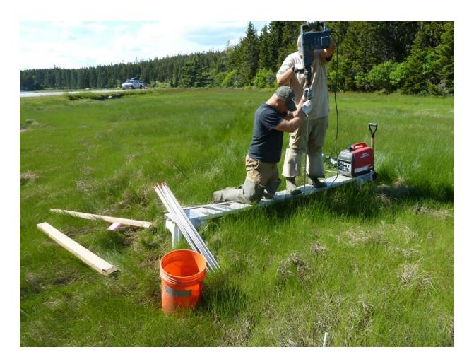
Figure 3.12. Driving rods. Note the bundle of rods on the end of the platform (Acadia NP, ME USA).
