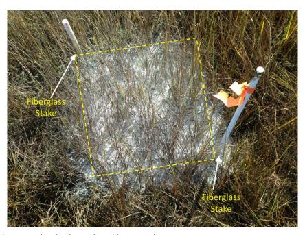
Figure 5.5. Feldspar marker horizon plot with two stakes.
