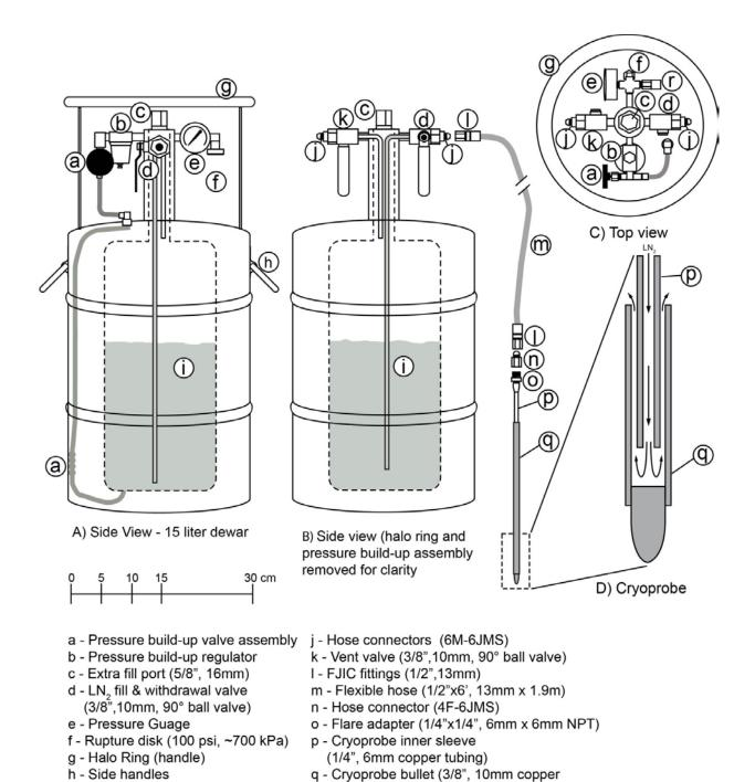
Figure 5.11. Schematic of the 15 liter dewar (from Callaway et al. 2013).
