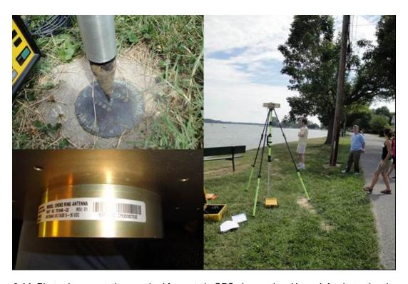
**Figure 6.14.** Photo-documentation required for a static GPS observation. Upper left: photo showing placement of GPS tripod over VPR of survey mark. Right panel: horizon photo showing deployment of entire GPS static assembly (GPS tripod, antenna, and receiver). Lower left: close-up of GPS antenna identification information.
