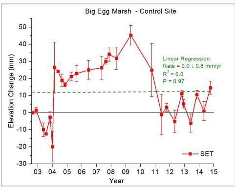
**Figure 18.** Elevation trends as measured by the SET method at Big Egg Marsh. Linear trends for the restored site cover a subset of the entire record (2005 – present) whereas trends for the control site cover the entire record (2002- present).
