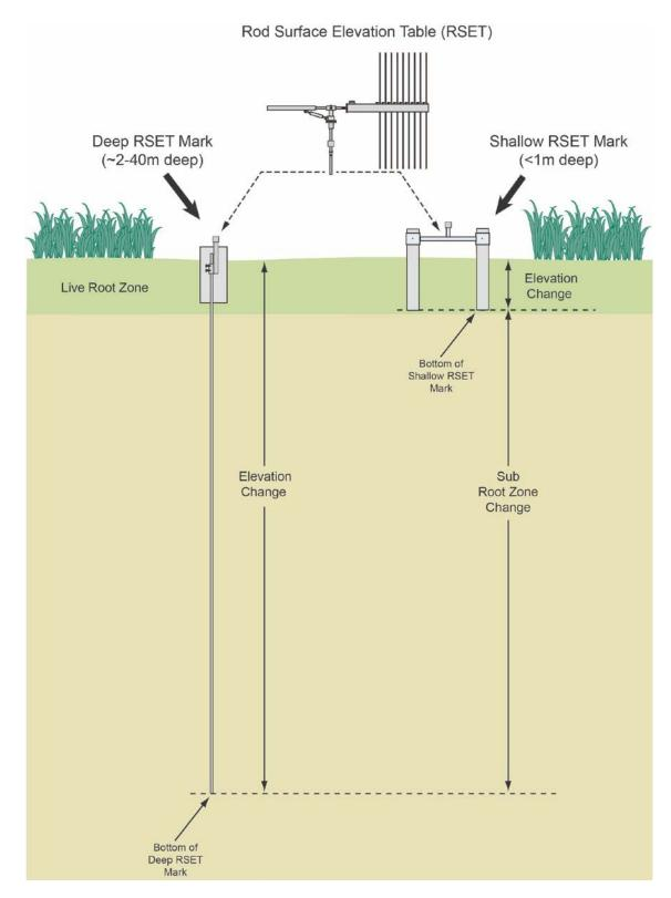
**Figure 6.** Conceptual diagram showing how the two RSET methods can be used together to partition vertical processes influencing wetland elevation between the live root zone and that portion of the substrate below the shallow RSET mark but above the base of the deep RSET mark (e.g., sub-root zone).
