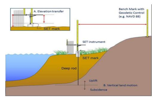
**Figure 6.4.** Surveying to an SET mark. Elevations can be transferred to a SET mark from a nearby bench mark by leveling. The elevation can then be transferred to the wetland surface measured by the SET (inset A) and to any nearby infrastructure of interest. A time series of repeated surveys can allow for the monitoring of vertical movement below the SET mark (B).
