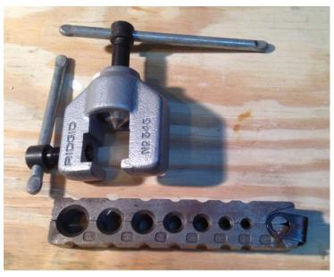
Figure 5.22. Tube flaring tool.
