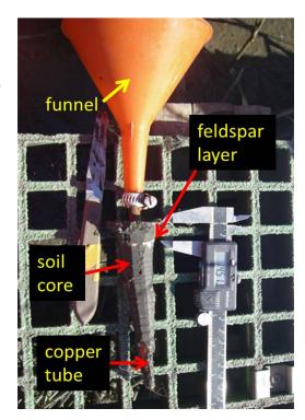
**Figure 5.9.** Frozen soil core taken with liquid nitrogen.
