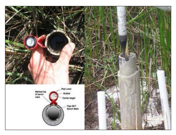
**Figure 6.5.** Finding the vertical point of reference (VPR) on an older, first generation SET pipe mark using a rod level (bubble gauge).
